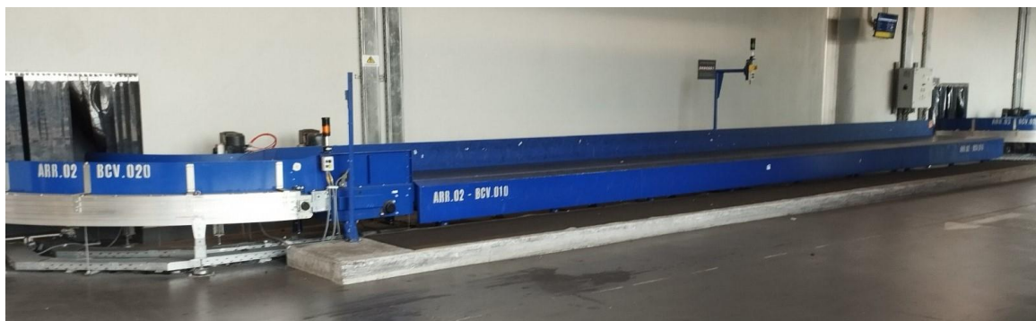
Figure 27: Infeed conveyor for arriving baggage
